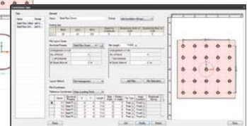
Pile Layout Dependent of Construction Method
