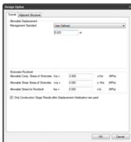
Allowable Displacement & Member Forces of Tunnels
